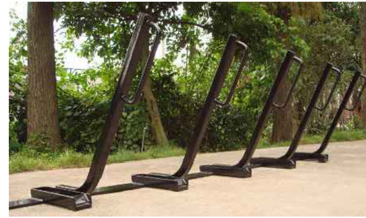
CLASS II (RACK/CORRAL) 3, 4, 5, 6, OR 8 UNIT MODULES AS REQUIRED TO MEET PARKING REQUIREMENTS AND SPACE ALLOWS. SHOWN: LIGHTNING BOLT BY SCH ENTERPRISES, OR SIMILAR. COLOR/FINISH: DARK BRONZE TGIC POLYESTER POWDER COAT (BLACK SHOWN)
